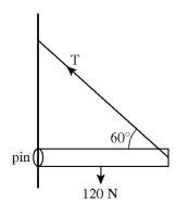
7. A uniform horizontal beam with a length of 6.0 m and a weight of 120 N is attached at one end to a wall by a pin connection so that the beam can rotate. The opposite end of the beam is supported by a cable attached to the wall above the pin. The cable makes an angle of 60.0° with the beam. What is the tension in the cable needed to maintain the beam in equilibrium?
